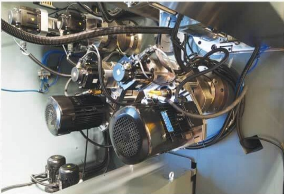
F1 BAR CNC Transfer Running 4m Circular, from 6 Edge and 8 Edge Material, \varnothing 6-30mm Diameter Interval, 4m Brass (Mach F1 Unit Group With 8 Station)
