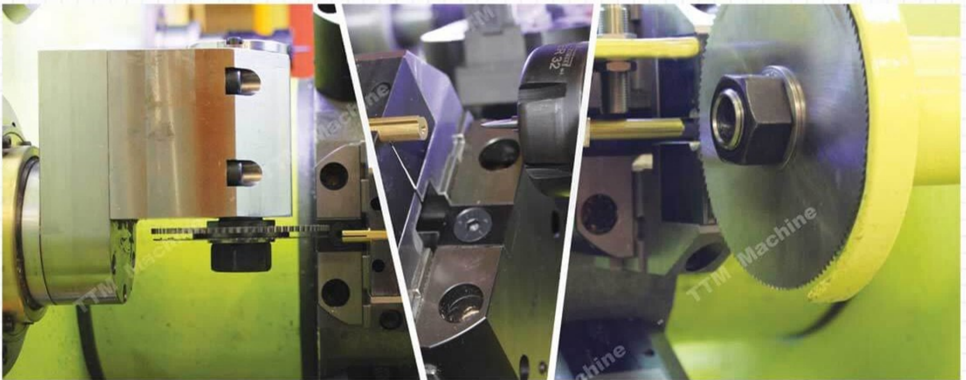
Mach unit group with 8 station drum - F1 bar CNC transfer
