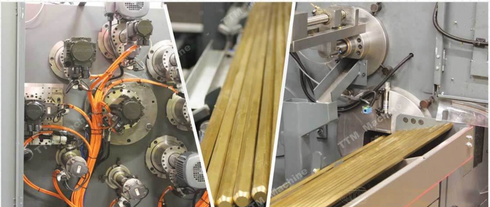
F1 BAR CNC Transfer Running 4m Circular, from 6 Edge and 8 Edge Material, \varnothing 6-30mm Diameter Interval, 4m Brass (Mach F1 Unit Group With 8 Station)
