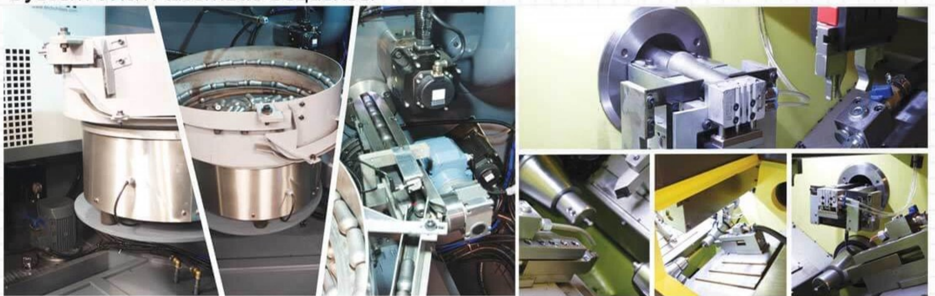
Full Automatic Part Feeder System With Automatic Sequencer
